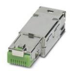
RJ45 connector, contact inserts: x , degree of protection: IP20, number of positions: 8, 1 Gbps, CAT5 (IEC 11801:2002), material: Zinc die-cast, connection method: IDC fast connection, connection cross section: AWG 26- 24, cable outlet: straight
