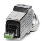
Push-pull connector (version 14), die-cast zinc, with RJ45 connector insert, 8-pos., with IDC fast connection technology, for 1 and 7-wire cores, 26 ... 24 AWG, for cable diameter of 5.5 mm ... 10 mm
