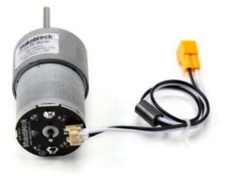
It can be connected with Makeblock Me Orion or Makeblock Me Dual Motor Driver V1 by adding the plug 3.96-2P on the stripped-end to control the motors.
