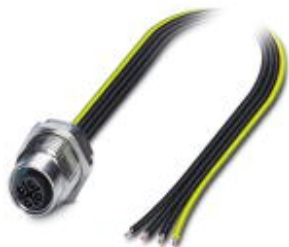
Flush-type connector, Power, 4-position, Socket, M12, S power, Rear mounting, M16 x 1.5, Individual wires, cable length: 0.5 m
