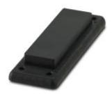
Cable feed-through plates, no. of conductors: 10, length: 154 mm, width: 56 mm, height: 20 mm, external cable diameter: 6x 2 mm ... 8 mm , color: black
