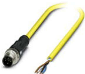
Sensor/actuator cable, 4-position, PVC, yellow, Plug straight M12 SPEEDCON, A-coded, on free cable end, cable length: 2 m
