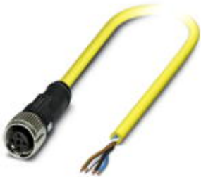
Sensor/actuator cable, 4-position, PVC, yellow, free cable end, on Socket straight M12 SPEEDCON, A-coded, cable length: 10 m
