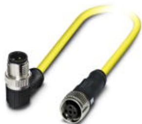
Sensor/actuator cable, 3-position, PVC, Plug angled M12 SPEEDCON, A-coded, on Socket straight M12 SPEEDCON, A-coded, cable length: 1.5 m
