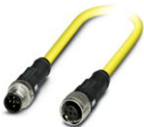
Sensor/actuator cable, 5-position, PVC, yellow, Plug straight M12 SPEEDCON, A-coded, on Socket straight M12 SPEEDCON, A-coded, cable length: 20 m
