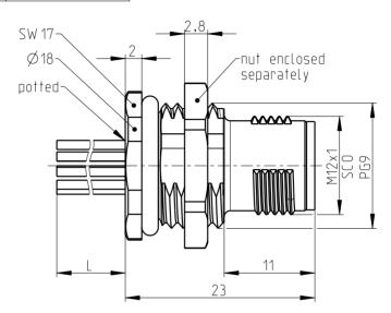
All specified data refers to the mounted M12 installation plugs  $\geq$  IP54 and requires that the connector pair be correctly plugged and locked. Influences from wires, cables or PCB mounting are also to be taken into consideration.
