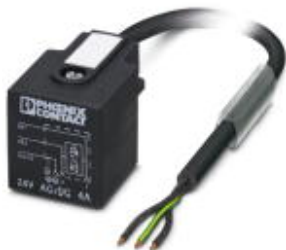
Sensor/Actuator cable, 3-position, PUR halogen-free, Black-gray RAL 7021, Free cable end, on A valve plug, with 1 LED, connected with Z diode, Cable length: 3 m
