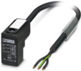
Sensor/Actuator cable, 3-position, PUR halogen-free, Black-gray RAL 7021, Free cable end, on C valve plug (8 mm), with 1 LED, connected with Z diode, Cable length: 1.5 m
