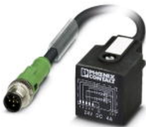
Sensor/Actuator cable, 5-position, PUR halogen-free, Black-gray RAL 7021, Plug straight M12, A-coded, on AD valve plug (pressure switch), with 2 LEDs, Cable length: 0.6 m
