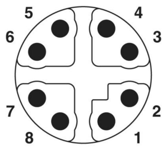
M12 Cat6<sub>A</sub>, 8-pos. connector pin assignment, pin side view
