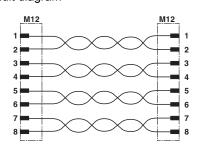
Contact assignment of the M12 plugs
