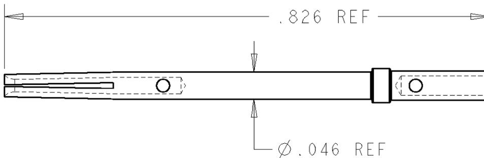
1. THIS SOCKET CONTACT IS A REPLACEMENT COMPONENT FOR USE ON QUADRAX SOCKET ASSEMBLY AS SHOWN ON THE FOLLOWING DRAWING(S): 1445693.
