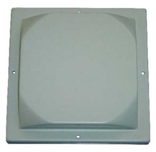
The UHF antennas ID ISC.ANT.U250/250-EU/-FCC are circular polarized antennas for operating frequencies in the UHF ranges 865-870 MHz (EU antenna) and 902-928 MHz (FCC antenna).
