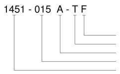
Coating (F = Gel Fill, Blank = No Coating) Port (T = Tube, N = Narrow Hole, W = Wide Hole) Type (A = Absolute, G = Gage) Pressure Range Model
