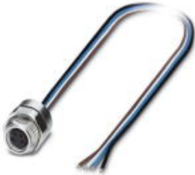
Sensor/actuator flush-type socket, 4-pos., M8, rear/screw mounting with M12 thread, with 0.5 m TPE litz wire, 4 x 0.25 mm²
