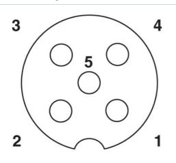
Pin assignment M12 socket, 5-pos., B-coded, view socket side
