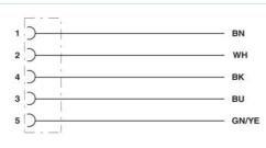
Contact assignment of the M12 sockets
