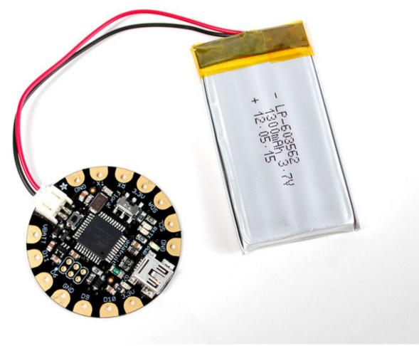
More advanced users may wish to use a rechargeable <u>lithium polymer</u> <u>battery</u> (http://adafru.it/258) for their smaller size and longer duration. These batteries pose added risk if abused, shorted, bent, crushed, or punctured. FLORA does not have onboard charging, so you would also need a separate <u>LiPoly charger</u> (http://adafru.it/259).
