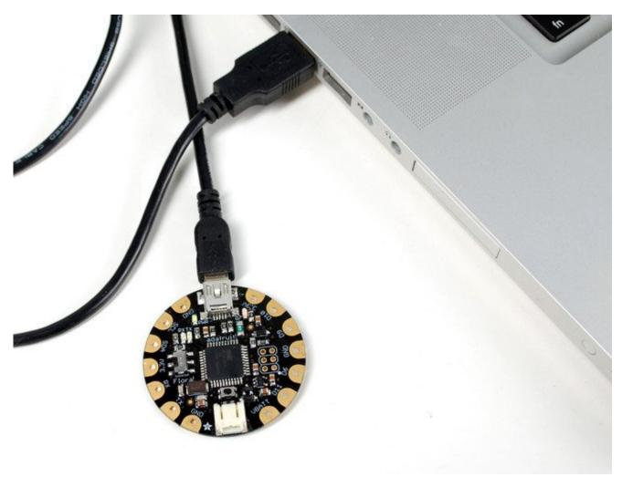
Next it's time to load up a program on your FLORA. There is an LED on board, so let's blink it! Plug in the USB cable and paste the following code into the Adafruit Flora IDE:
