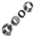
Metal screw connection up to 5 bar, thread length: 6 mm, cable diameter: 9 - 13 mm, WAF 22, screw connection: M20
