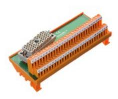
ELCO contacts inserts are used in electrical power plants, refineries and a variety of process applications – wherever stable and reliable signal transmission is required. The ELCO connector features both a reliable connection system and a high signal capacity.
