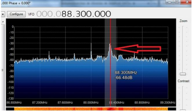
With the latest versions of SDR-Sharp it will automatically detect and decode RBDS/RDS data that is sent along with FM radio
