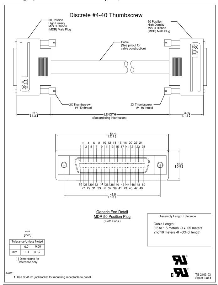
.050" High Speed Video Data Transmission System, 50 Position
