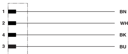
Contact assignment of M8 plugs/sockets
