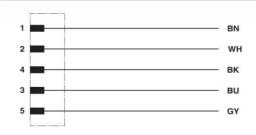
Contact assignment of the M12 plug
