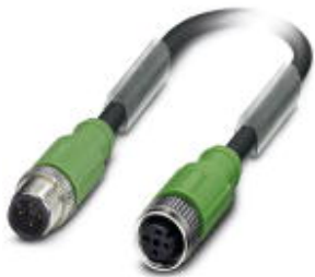
Sensor/actuator cable, 4-position, PUR halogen-free, black-gray RAL 7021, shielded, Plug straight M12, A-coded, on Socket straight M12, A-coded, cable length: 3 m
