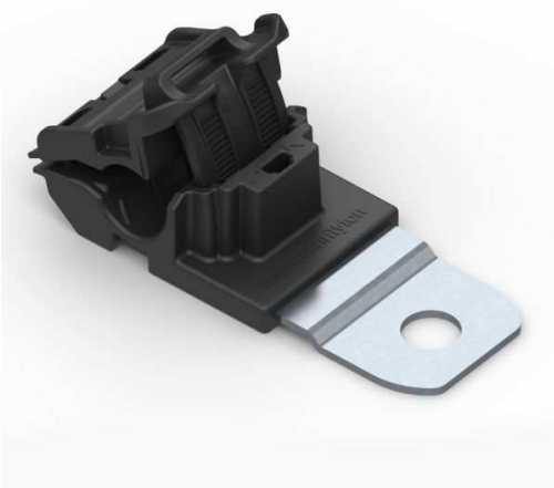
Ratchet P-Clamp, .24"—.54" Bundle Dia, 180° Medium, .33" Hole Dia, PA66HIRHSUV/SS304, Black, 200/ctn
