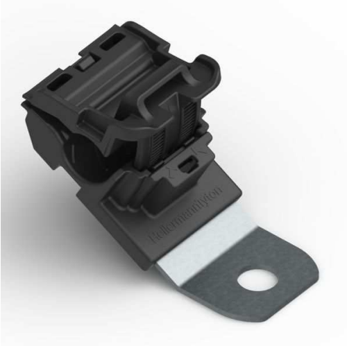
Ratchet P-Clamp, .24"—.54" Bundle Dia, 30° Long, .26" Hole Dia, PA66HIRHSUV/SS304, Black, 200/ctn
