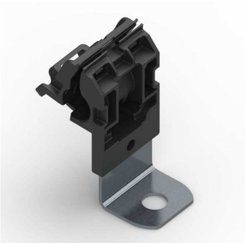
Ratchet P-Clamp, .24"—.54" Bundle Dia, 90° Long, .26" Hole Dia, PA66HIRHSUV/SS304, Black, 200/ctn
