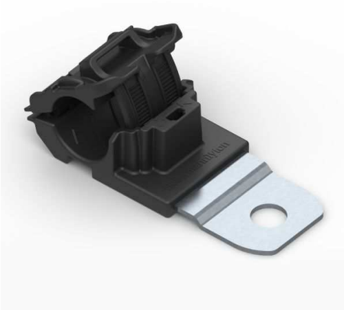
Ratchet P-Clamp, .52"—.77" Bundle Dia, 180° Medium, .41" Hole Dia, PA66HIRHSUV/SS304, Black, 200/ctn
