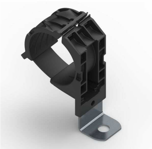
Ratchet P-Clamp, 1.38"–2.01" Bundle Dia, 90° Short, .41" Hole Dia, PA66HIRHSUV/SS304, Black, 160/ctn
