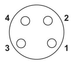
Pin assignment M8 female connector, 4-pos.
