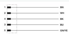
Contact assignment of the M12 plug
