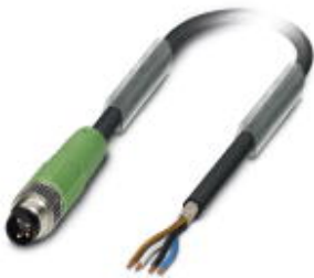
Sensor/actuator cable, 4-position, PUR halogen-free, black-gray RAL 7021, shielded, Plug straight M8, on free cable end, cable length: 3 m
