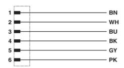
Contact assignment of the M8 plug
