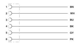
Contact assignment of M8 socket
