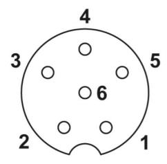
Pin assignment M8 socket, 6-pos.
