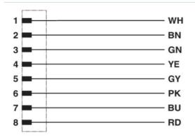
Contact assignment of the M12 plug
