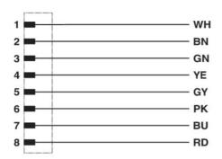
Contact assignment of the M12 plug
