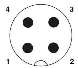
Pin assignment M12 Y plug, 4-pos., A-coded, view plug side
