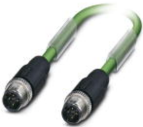
Bus system cable, PROFINET CAT5 (100 Mbps), 4-position, PVC, green RAL 6018, shielded, Plug straight M12, D-coded, on Plug straight M12, D-coded, cable length: 15 m
