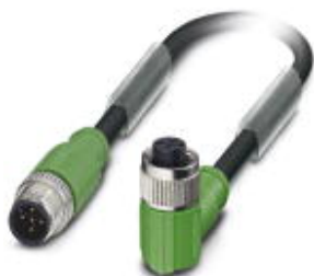
Sensor/actuator cable, 5-position, Variable cable type, shielded, Plug straight M12, A-coded, on Socket angled M12, A-coded, cable length: Free input (0.2 ... 40.0 m)
