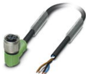
Sensor/actuator cable, 4-position, PUR halogen-free, black-gray RAL 7021, free cable end, on Socket angled M12 SPEEDCON, A-coded, cable length: 3 m
