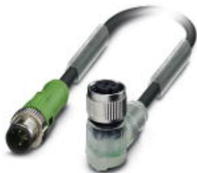
Sensor/actuator cable, 3-position, Variable cable type, Plug straight M12 SPEEDCON, A-coded, on Socket angled M12 SPEEDCON, A-coded, with 2 LEDs, PIN 2+4 bridged, cable length: Free input (0.2 ... 40.0 m)
