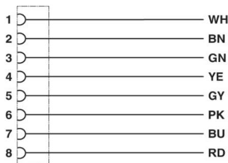
Contact assignment of the M12 socket
