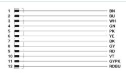
Contact assignment of the M12 plug
