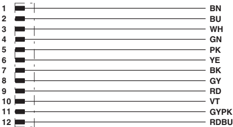
Contact assignment of the M12 plug
