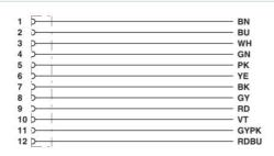
Contact assignment of the M12 socket
