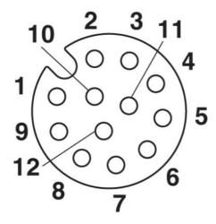
Pin assignment M12, 12-pos., female side view
