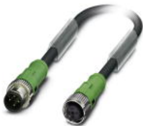
Sensor/actuator cable, 4-position, PUR, black-gray RAL 7021, Plug straight M12 SPEEDCON, A-coded, on Socket straight M12 SPEEDCON, A-coded, cable length: 2 m
