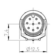
All specified data refers to the mounted M12 installation plugs  $\geq$  IP54 and requires that the connector pair be correctly plugged and locked. Influences from wires, cables or PCB mounting are also to be taken into consideration.
